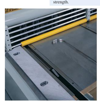
Gauge stops located on 24" centers travel 24" front to rear in unison. This yields a total gauging range of 72", 120" or 144" with the operator selecting the proper stop. Indicator on the display panel designates which stop to use depending on the dimension programmed. Air finger option elevates only the correct finger.
